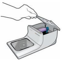
2 Push the blue cartridge release lever to unlock the purple cartridge latch.
